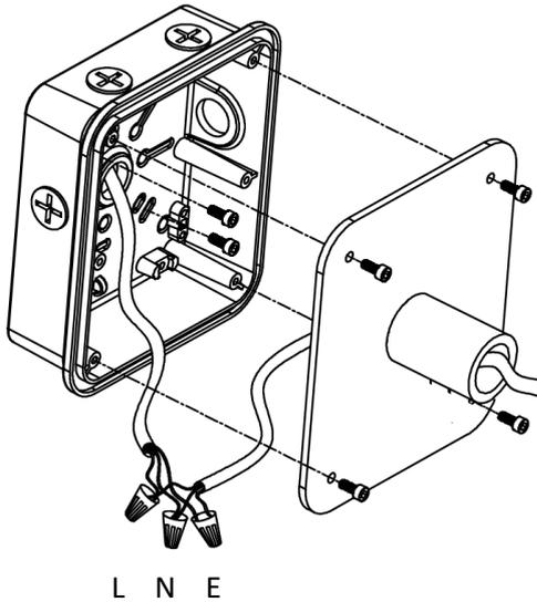
3. Fix the base of the connection box to your surface using by drilling holes in the bottom of the base.
